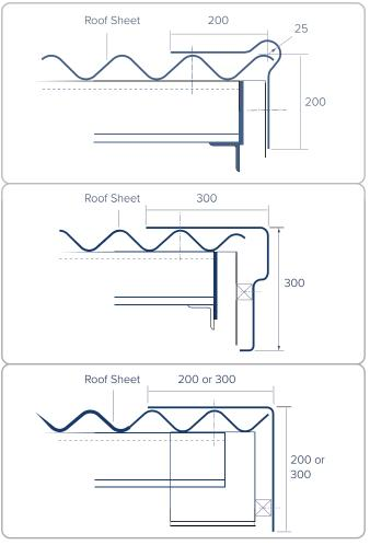
\*No fixing should be within 50mm of any edge of the bargeboard
